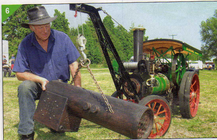
6 Ray Darvell checks out the lifting capability of his 4in. Foster crane engine.
